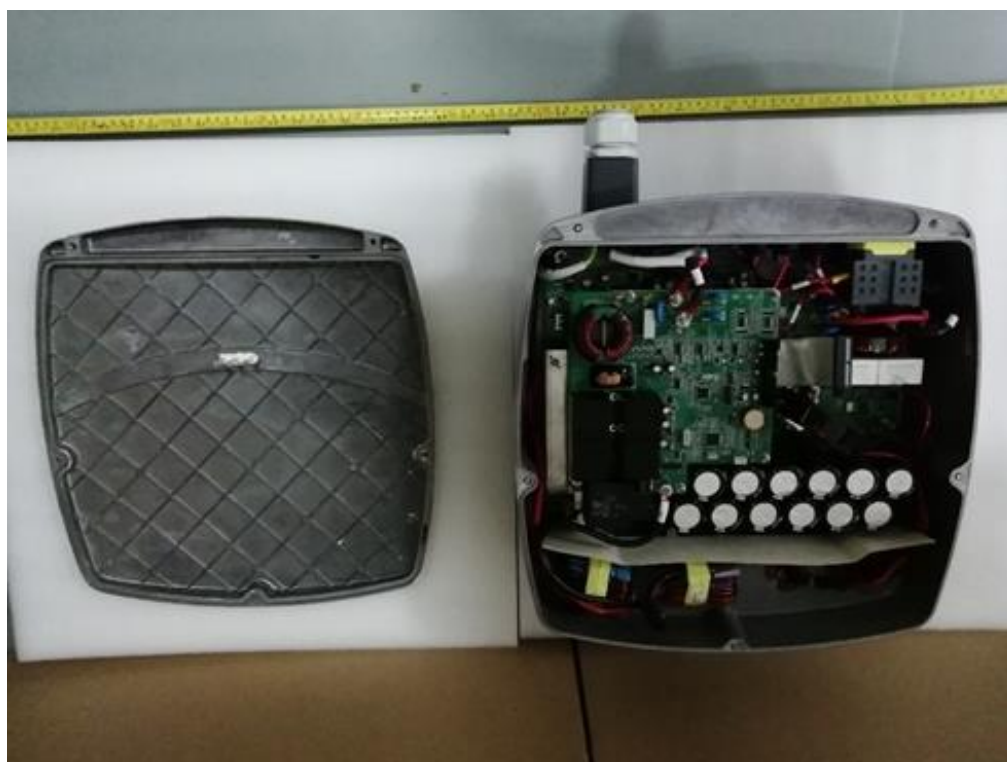
Internal view of inverter
